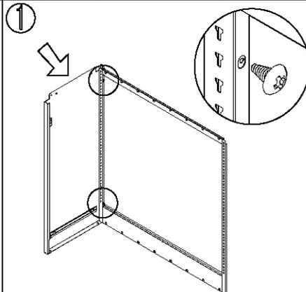
1 Connect the left side plate with back plate by self-tapping screws(5x12).
