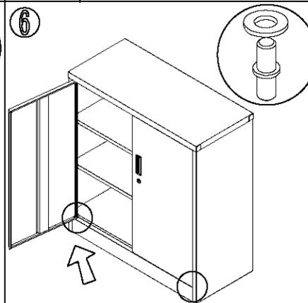
6 Install the door, and adjust each parts till fit well after installation.
